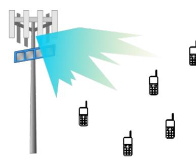
E.g. A multi-antenna base station broadcasts an OFDM signal containing a control message to a set of connected devices through a random beam. A radar receiver, co-located with the base station, listens to the echo of the transmitted signal and processes it to detect the presence of new users, and their position in space.
