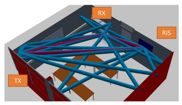
Using the ray-tracing module of the simulation framework SiMoNe, the performance of IRS-assisted communication links can be analyzed. In the shown case, SiMoNe's integrated 3D-visualization framework shows the complex multipath propagation in a small meeting room scenario featuring an IRS-assisted connection between a transmitter and a receiver as it might be used to enhance the physical layer security by circumventing possible eavesdropper spying on the direct link.
