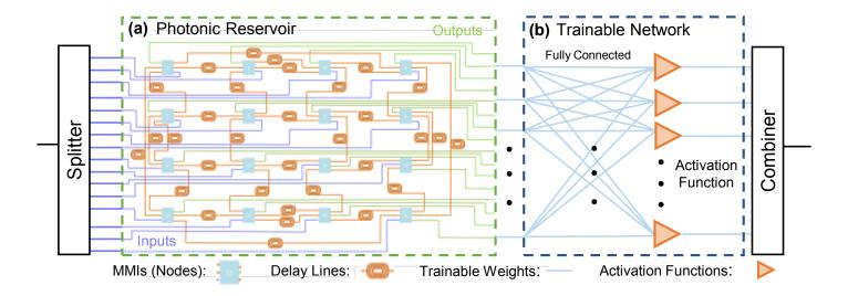
The schematics of the optical reservoir of a 4-port architecture following a 1-fully-connected layer of training network including complex weight functions and Indium Phosphide (InP) semiconductor optical amplifier (SOA) activation functions.
