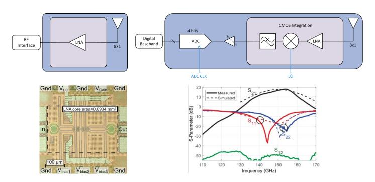
Proposed demonstrator design; Fig. 1. The first demonstrator consists of an 8x1 antenna array with an integrated LNA, the RF-interface will be realized using waveguides; Fig. 2. Final demonstrator, all circuit components integrated into one monolithic IC, LO and ADC CLK will be supplied externally. Fig. 3 Simulated and measured S-Parameters and die photograph of the LNA [1]
